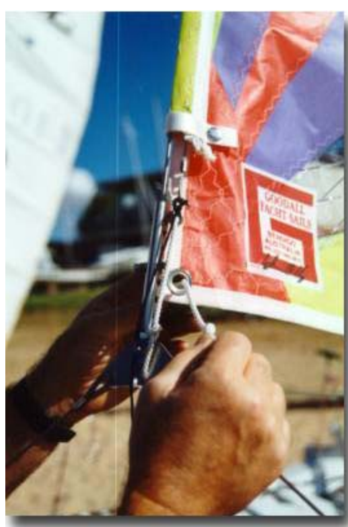
4. Thread the knotted tail through the tack eye of the jib. Again, the length of the rope needs to be carefully adjusted on the first occasion a new jib is used.
