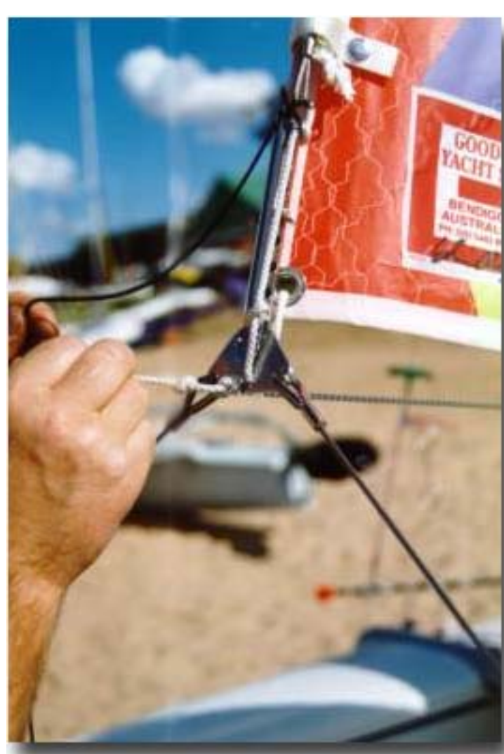
6. The chosen knot is slipped into the slot on the bridle plate, all that remains is to tidy up the loose ropes and go sailing. The best place for the loose tail is looped back under itself. Adjustment is achieved by selecting the appropriate knot.
